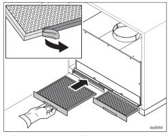
Take the grease filters out and remove any protective foil. Replace the grease filters.
